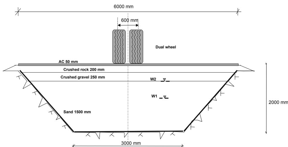
Figure 2.11. Cross-section of the structure /Korkiala-Tanttü et al. 2003b/.
