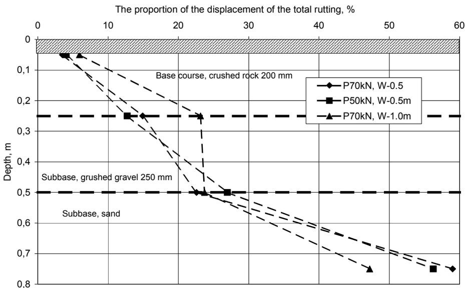
Figure 3.9. Proportion of deformations in different layers of the total rutting / Korkiala-Tanttu et al. 2003b /.
