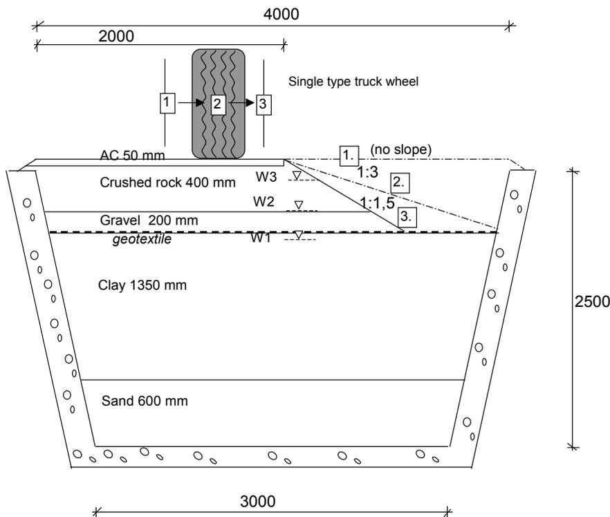
Figure 2.7. Cross-section of low-volume structure (no slope, 1:3 and 1:1.5 slopes) /Korkiala-Tanttu *et al*. 2003a/.
