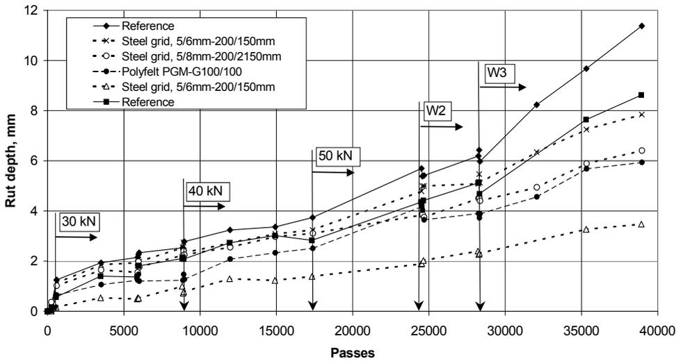
Figure 2.17. Rutting of the surfaces of the structures
