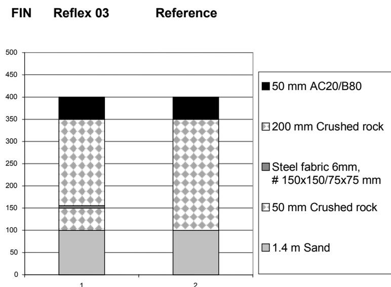
Figure 2.1. Test structure, Reflex 03 /Pihjalamäki et al. 2002/.
