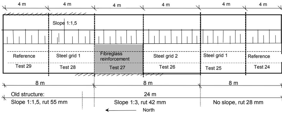
Figure 2.15. Test structures and their state before rehabilitation.
