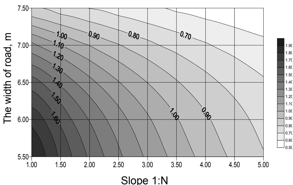
Figure 3.7. GEOM factor as a function of slope steepness and road width /Korkiala-Tanttu et al. 2003a/.
