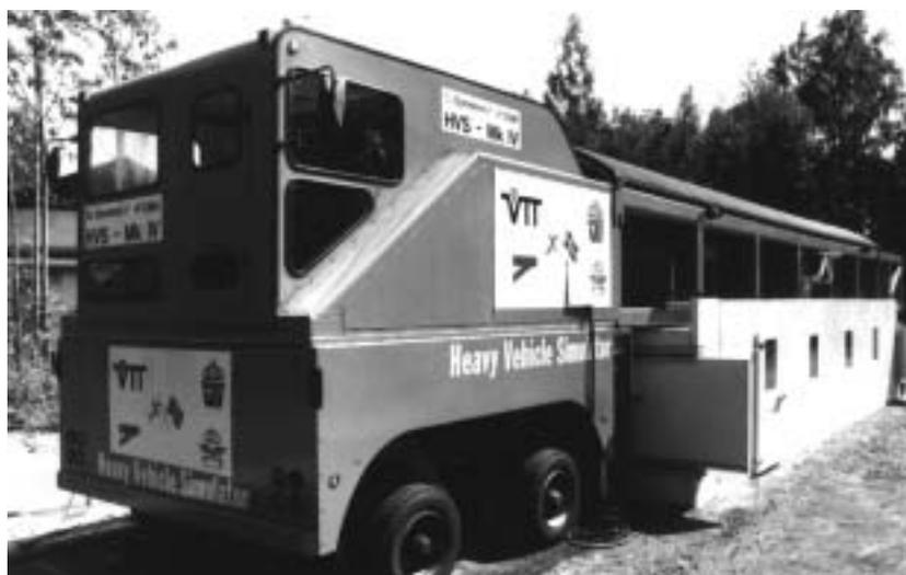
Figure 1.1. HVS-NORDIC accelerated pavement testing facility.
